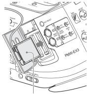
Insert so that the cable extends upward.
